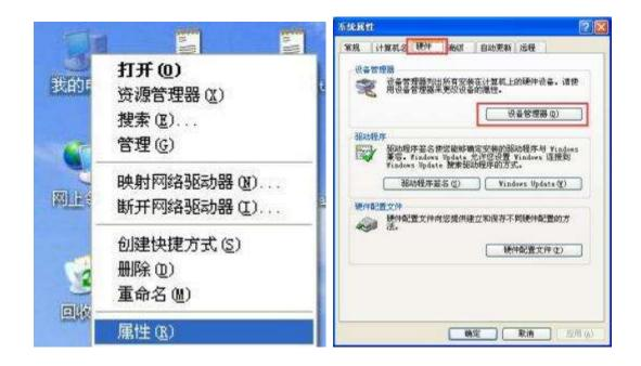
(2) Plug in the USB cable and connect the spectrometer to the computer, and the uninstalled USB device with a yellow question mark or exclamation mark (or display the name "USB Device") will be displayed in the device manager,right-click the device name - "Update Driver" to enter the hardware update wizard;
