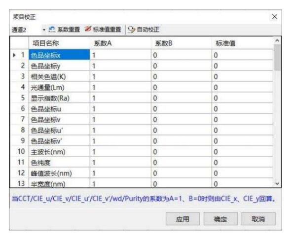
**Coefficient Reset:** Resets coefficient A to 1 and coefficient B to 0;
